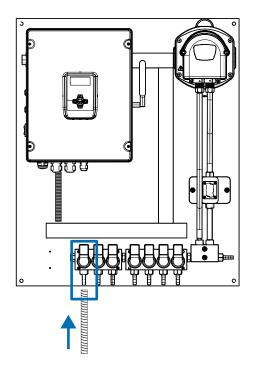
Connect the water supply to the water inlet connection seen on the unit here.
