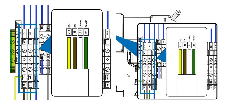
To connect the expansion channel to the unit, connect X2 on the main machine to X1 on the expansion channel.
