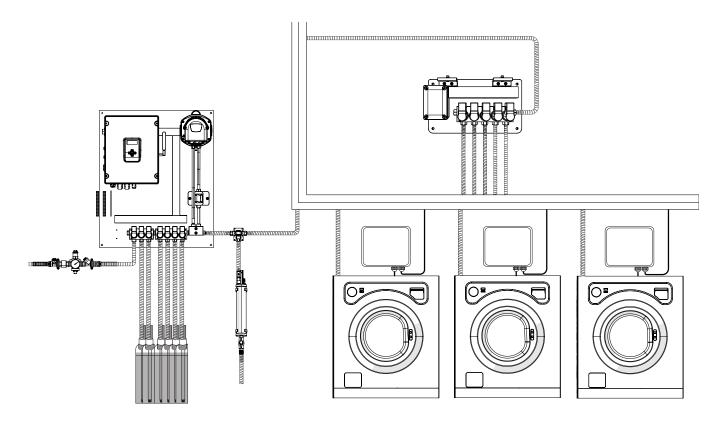
This image reproduces the 'Standard' setup of a Multiplex unit with one channel and an external distributor (your setup will vary based on model), understanding "Channel" as a group of products that are injected into the same manifold and directed to a distributor (washing machines) or an injection (tunnel).
