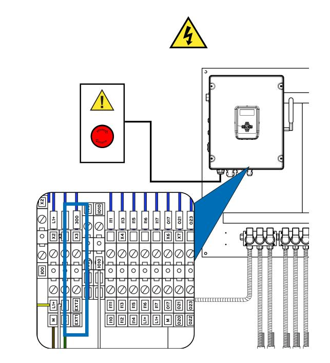
To connect an emergency stop button to your unit, you can use the EXT1 and EXT2 connectors slot shown above.
