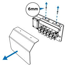
To mount your external distributor unit, please remove the cover using a **6mm** hex bolt.
