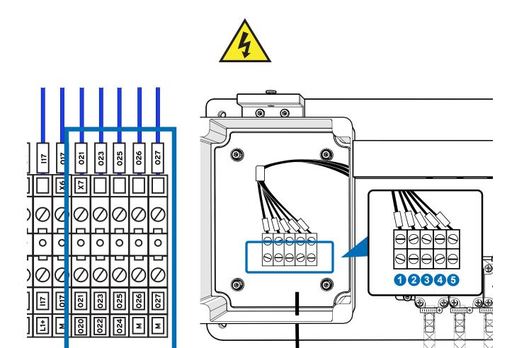
Use a 7x1mm^2 cable for the connection between the control cabinet and the distributor. Connect the distributor to terminal block X7. Each terminal connection corresponds to the outlets numbered from left to right, with the number dependent on the order. Below is the wiring diagram for the main unit.
