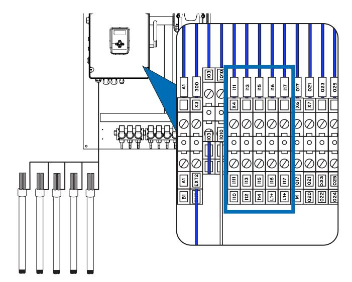
To connect the external suction lances to the machine, utilize inputs I10 to I17, as indicated above.
