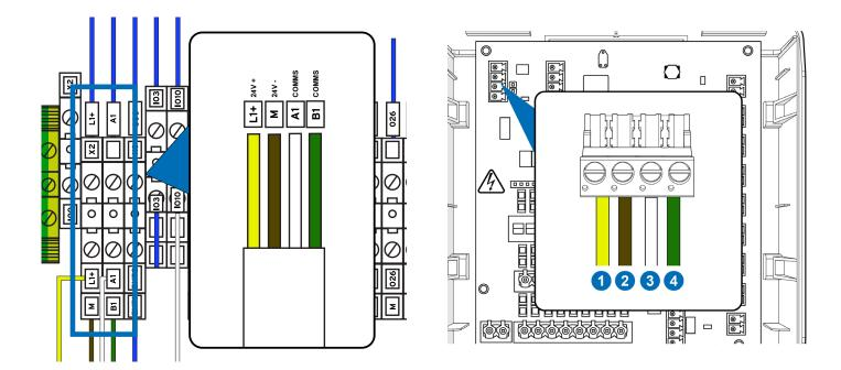
To connect the external communication box to the unit, connect terminal X2 on the main machine to terminal X1 on the communication box. Each communication box can serve up to two washing machines in series.
