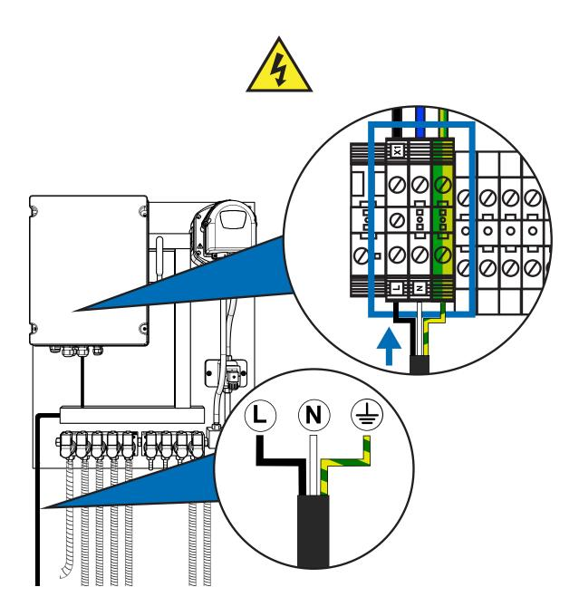
For the power supply of the equipment you must use **3x16 AWG cable**. Insert the cable through the channel located at the bottom left and use one of the cable glands to insert it safely inside the control cabinet. Connect to the terminals identified with **X1** found on the lower left of the connections.
