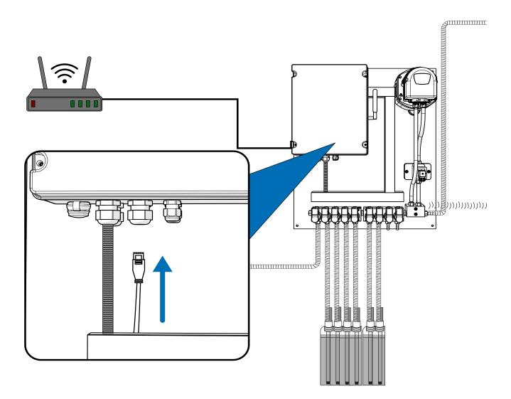
To connect your unit to the internet, simply plug an Ethernet cable into any router through the connector located on the bottom of the main box.
