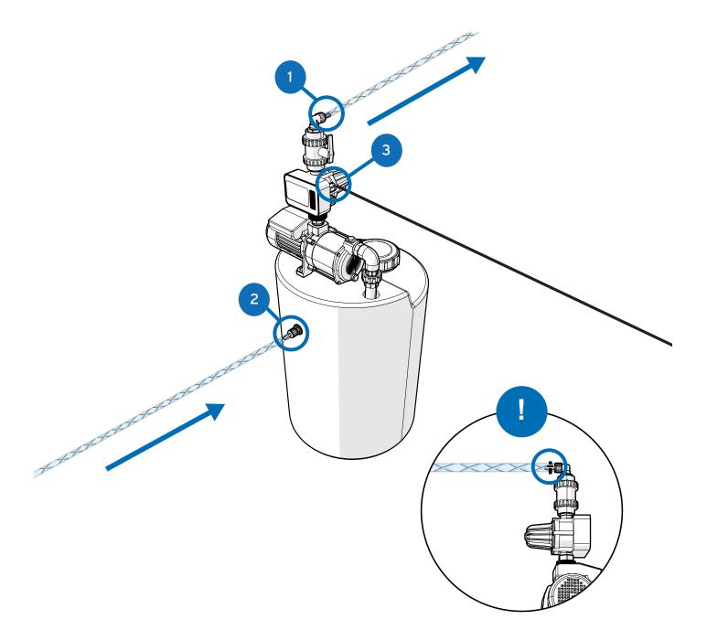
Please note that the unit requires a flow rate of min 68 fl oz per min - max 339 fl oz per min and a dynamic pressure range of 28 PSI (min) - to 44 PSI bar (max). A booster tank is recommended whenever a consistent supply is not available.
