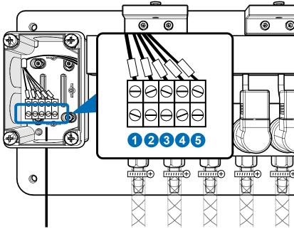
Use a **7x18** AWG cable for the connection between the control cab inet and the distributor. Connect the distributor to terminal block **X7**. Each terminal connection corresponds to the outlets numbered from left to right, with the number dependent on the order. Below is the wiring diagram for the main unit.
