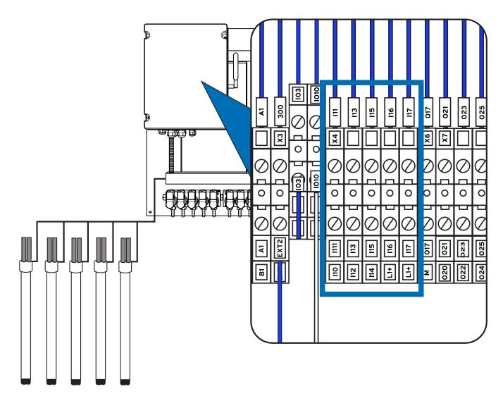
To connect the external suction rods to the machine, utilize inputs I10 to I17, as indicated above.
