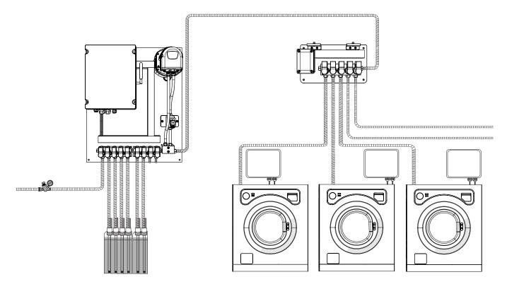
This image reproduces the 'Standard' setup of a Multiplex unit with one channel, understanding "Channel" as a group of products that are injected into the same manifold and directed to a distributor (washing machines) or an injection (tunnel).
