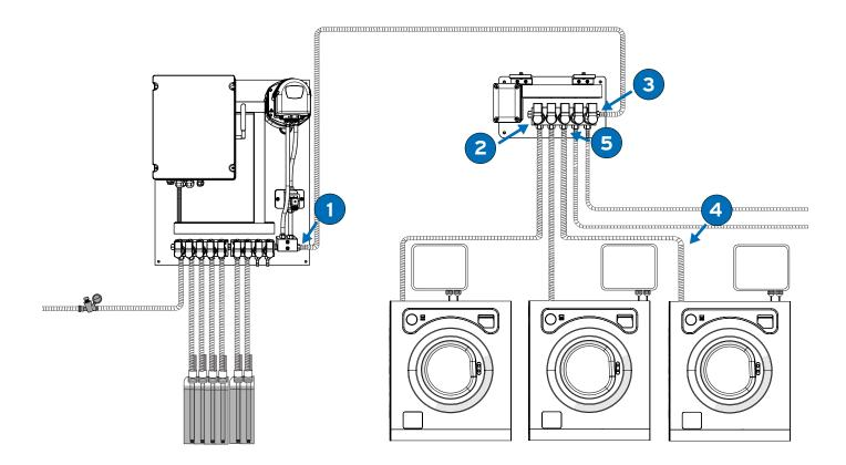
To connect equipment, distributor and washers, use 3/8" ID x 1/2" OD braided PVC pipe and stainless steel clamps.
