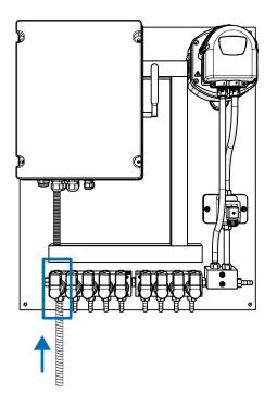
Connect the water supply to the leftmost solenoid valve on the central panel of the unit.
