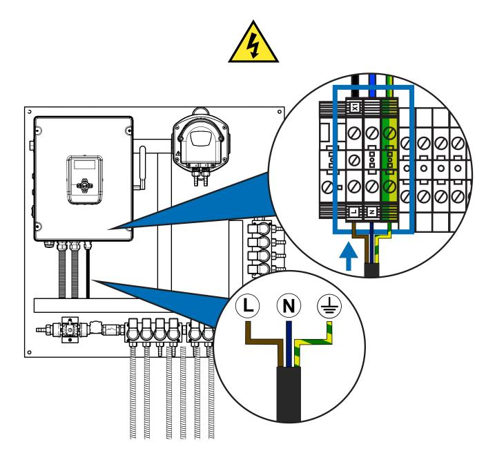
For the power supply of the equipment you must use **3x16 AWG cable.** Insert the cable through the channel located at the bottom left and use one of the cable glands to insert it safely inside the control cabinet. Connect to the terminals identified with **X1** found on the lower left of the connections.
