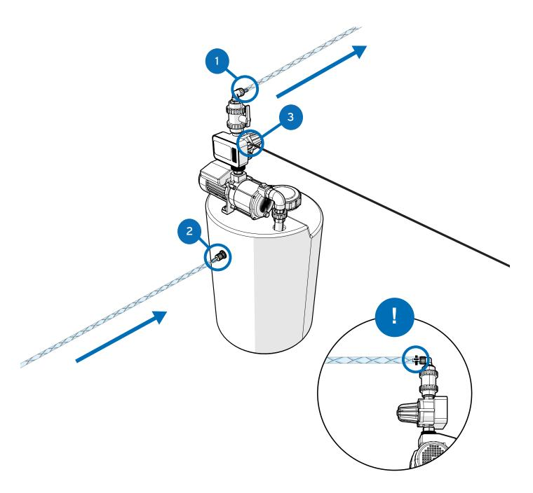
Please note that the unit requires a flow rate of min 68 fl oz/min - max 339 fl oz/min and a dynamic pressure range of 1.5 bar (min) - to 3 bar (max). A booster tank is recommended whenever a consistent supply is not available.
