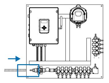
Connect the water supply to the water inlet connection seen on the unit here.
