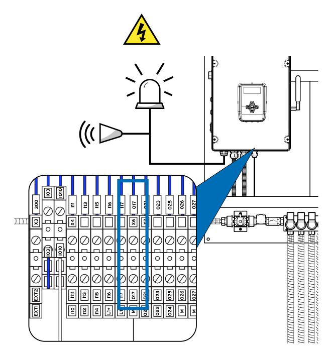
To connect an external alarm or warning light to the system, utilize slot X6 as depicted above.
