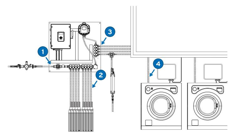
To connect equipment, distributor and washers, use 3/8" ID x 1/2" OD braided PVC pipe and stainless steel clamps.
